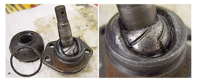
This is a new style upper ball joint. Unlike the older ones this one has grooves on the ball so grease can work it's way to all surfaces of the ball. These ball joints all have grease fittings and can last over 100,000 miles. The one pictured had 58,000 on it.
