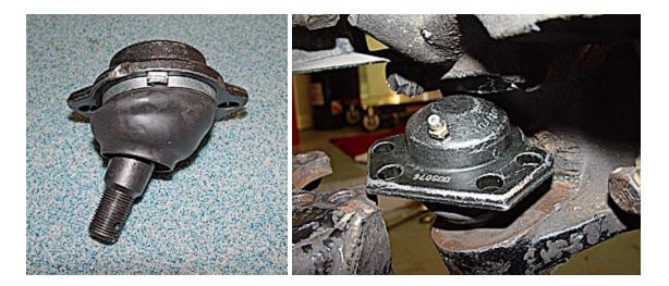
Bend the new joint all the way over to the side. Twist the joint about 90 degrees and it will drop into the hole in the lower geared hub. The first time I tried to put one in I tried to get it in straight and it got caught up and jammed on a small ridge which is part of the geared hub casting. The lower joint goes under the lower control arm.
