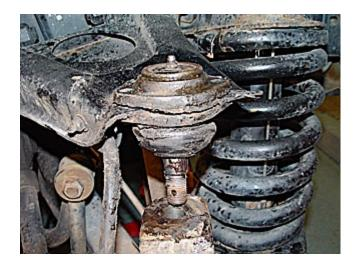
You can now pull the old ball joint up and out of the upper control arm.
