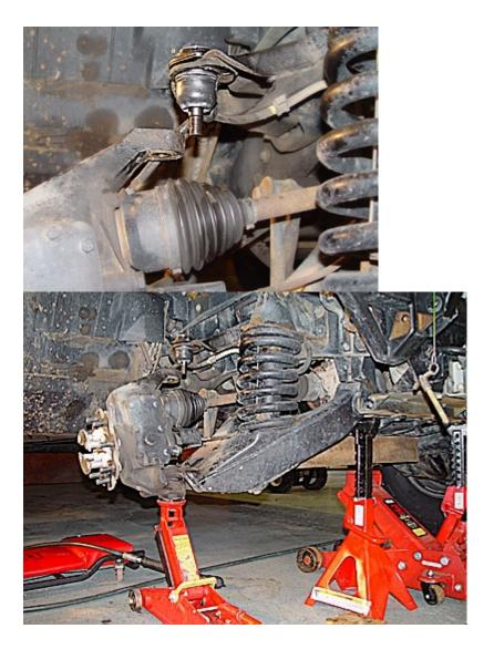
Clean all debris around the hole in the hub and the upper control arm. Drop the new ball joint into the hole in the upper control arm. Make sure that the rubber boot does not get pinched in the control arm hole. Push it down clear through.
